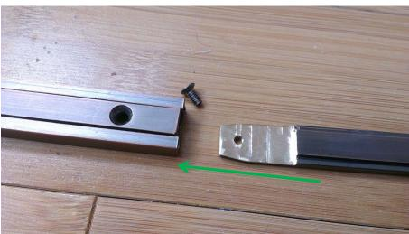
Using a normal B85C450BZ bolt ensure the case of the bolt is orientated into the non-key locking position.
