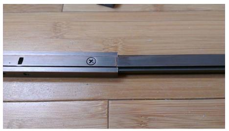
Insert the machined nose part of the bolt into its mating part and join with the screw provided.
